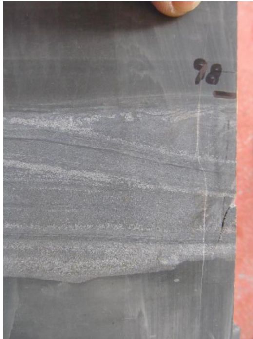
A calcite-mineralized, high-angle extension fracture cuts a coarse-grained calcarenite limestone bed, extending for short distances upward and downward into the adjacent mudstones. Fingertip at the top of the photo for scale.
