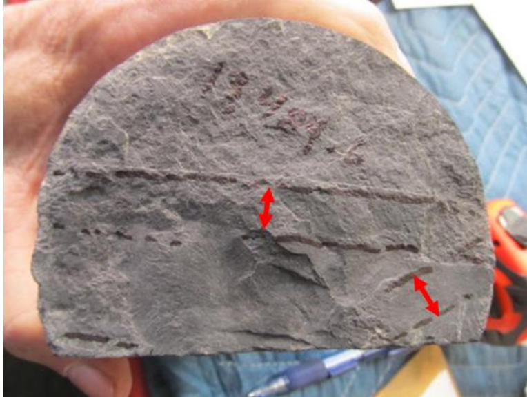
Measurable spacings (red arrows) between two pairs of narrow, closely-spaced, calcite-mineralized high-angle extension fractures (highlighted by dashed black lines drawn adjacent to the fractures), exposed on a bedding plane.
